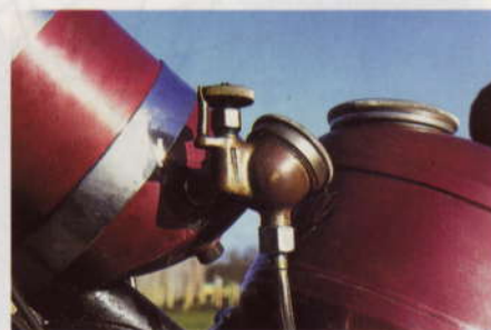
Two-stroke oil flows from separate tank. Amount is set by hand operated drippers
