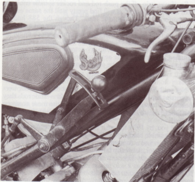
(Top) In Stanford Hall's stately grounds, Titch gets awheel. (Bottom) The two-compartment tank has been converted to hold only petrol, the old oil tank now a reserve. Gatechange, here in neutral, reveals there are only three gears which the owner regards as sufficient. Remember, it's a six-hundred with the torque of a four. Water circulation is thermo-siphon (no pump).
